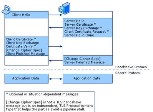
The Handshake protocols manage this process of exchanging key generation material, and it uses the Handshake Protocol.
